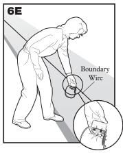
If the Collar Receiver does not beep at the desired range, adjust the Range Adjuster knob to the desired setting. Turning the Range Adjuster knob clockwise increases the Boundary Width while turning it counterclockwise decreases it. Repeat this activity as needed until the Collar Receiver beeps at the desired distance from the Boundary Wire.
