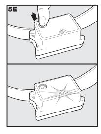
The Correction Levels increase in strength from 1 to 5. Pushing the Correction Level Button while the Collar Receiver is on level 5 will cause the Collar Receiver to revert to level 1. Refer to the Function and Response Table to choose the Correction Level that best fits your pet.
